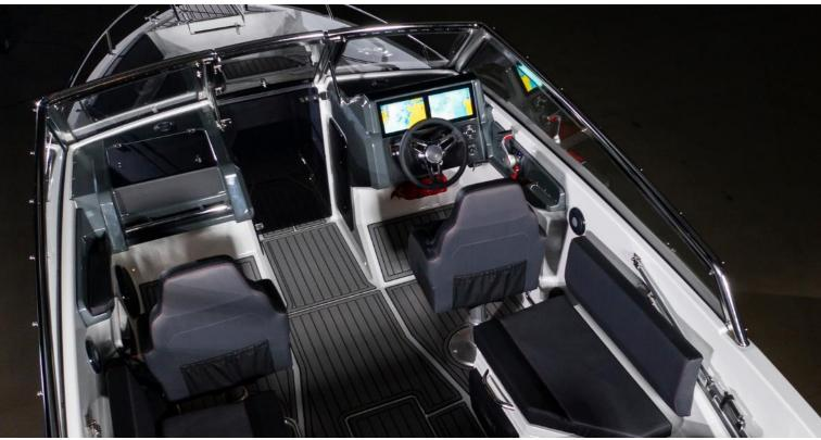
High and long windshield with a stylish stainless-steel frame, provides excellent protection for driver and passengers.
