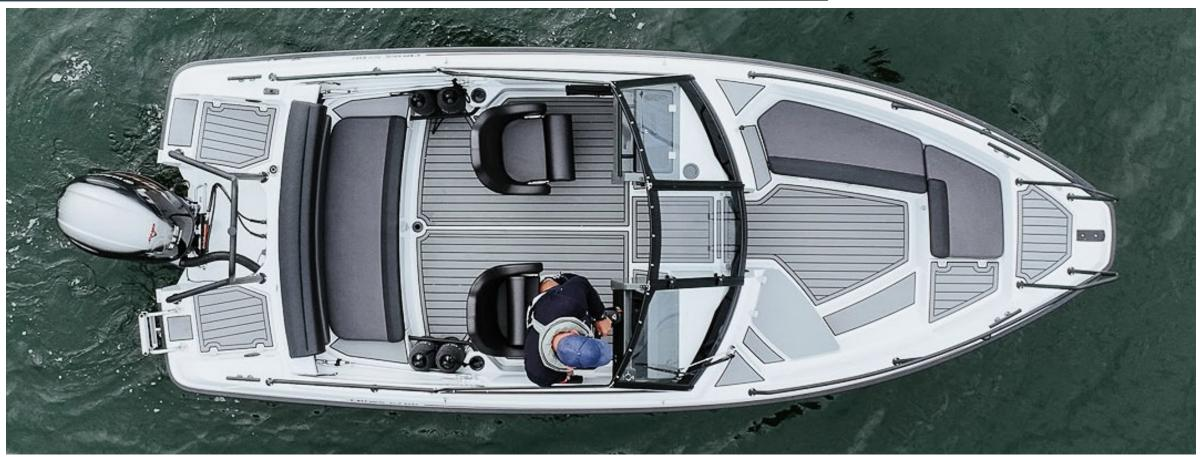
The comfortable Softdeck as standard – a durable and non-slippery deck material.
